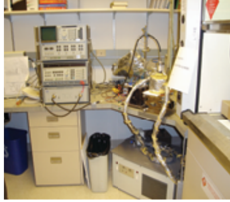
Dielectrik probu ve HP 85108 Network analizörü Hewlett-Packard
